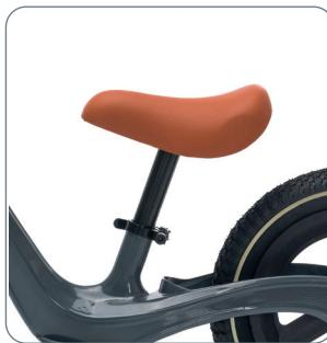
Seat installation: Place the seat into the frame, adjust the appropriate height, and tighten the quick release screws.
