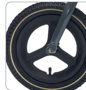
Insert the front wheel gasket and tighten the screws.
