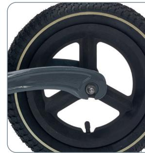
Insert the rear wheel gasket and tighten the screws.
