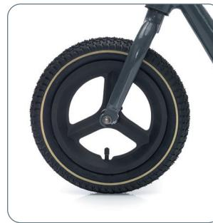
Mount the front wheel: First, place the front wheel onto the front fork.
