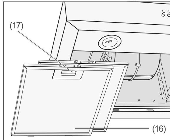
2. Open the lock (17) and carefully remove the grease filter (16).
