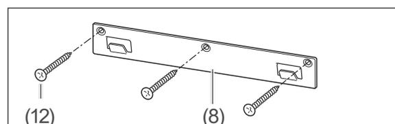
2. Screw the wall bracket (8) for the exhaust hood into the dowels using three round-head screws (12).
