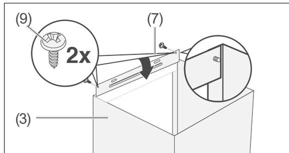
2. Place the retaining plate (7) onto the lower flue screen (3) so that it lines up with the chamfers on the inside. (Screws and elongated holes should point upwards).
