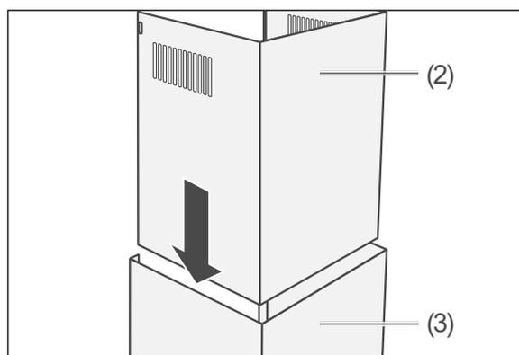
4. Push the upper part (2) of the flue screen halfway into the lower part (3) of the flue screen.
