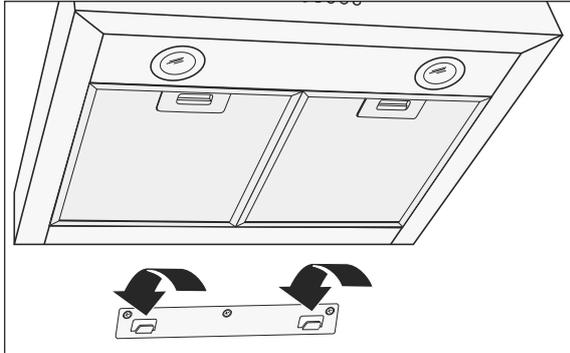
3. Hook the exhaust hood onto the wall bracket (8).
