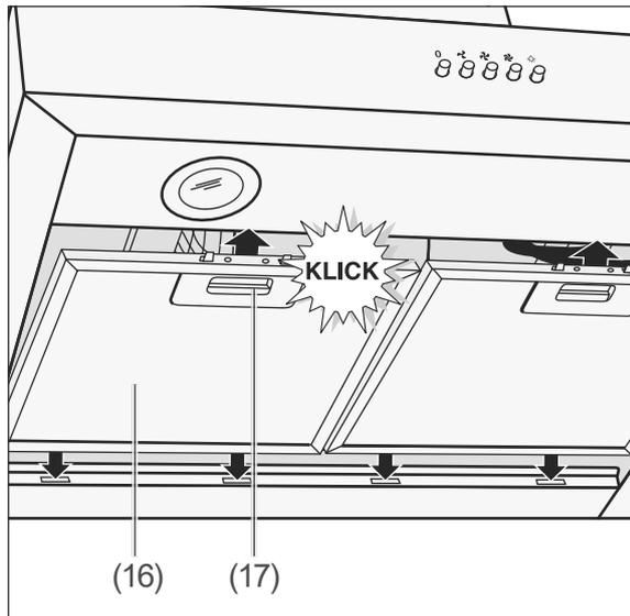
5. Place a grease filter (16) with the pins into the openings.
