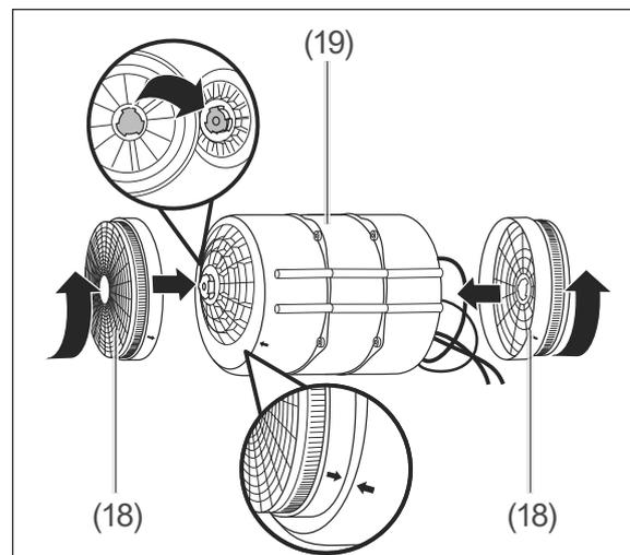
5. Place the new activated charcoal filters (18) to the right and left of the motor (19) as shown and tighten them in an anti-clockwise direction. Allow the locks to snap into place.
