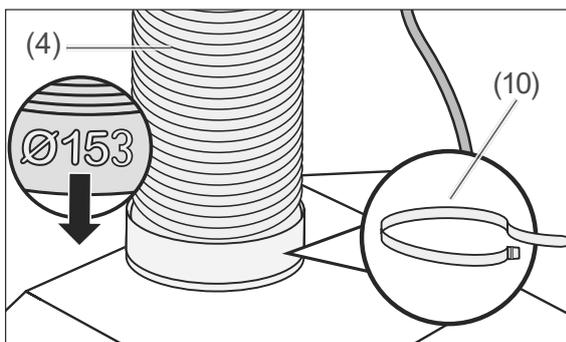
1. Insert the end of the exhaust hose (4) with the larger diameter (153 mm) into the connection with the check valve.
