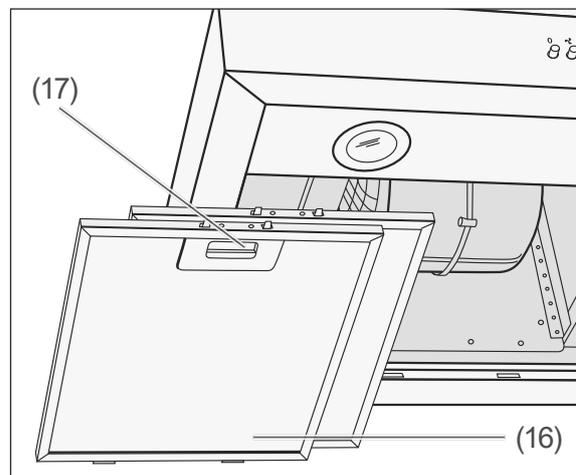
2. Open the lock (17) on one grease filter (16) and carefully remove the grease filter.
