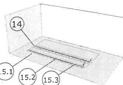
Make sure that all panels that you need to apply glue to are clean from dust,dirt and oil and then apply glue on them.
