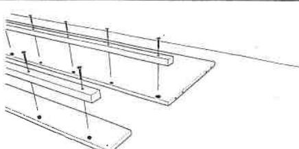
Gently apply pressure on the surface of the panels and secure them with screws.
