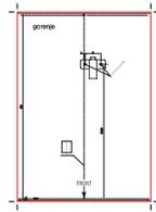
2. Make the marks on the bottom of the cabinet according to marks »A« on the template.
