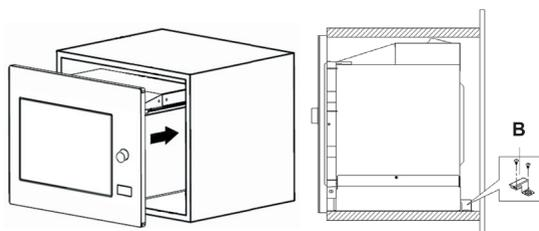
5. Open the door, fix the oven to the cabinet with screw (D), at the installation hole. Then fix the plastic cover to the installation hole (E).
