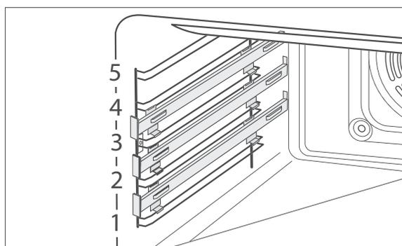
Please note that the baking tray should be slightly below the rack height marking when it rests on telescopic rails (see Fig. left).
