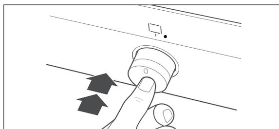
The function selectors can be pushed in to protect them from hot steam and contamination during operation.
