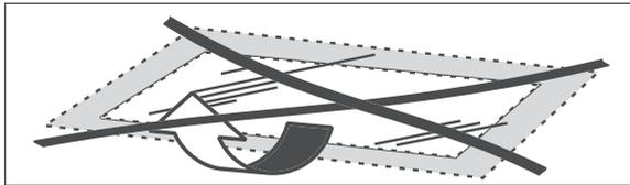
10. Reposition the upper pane in the mounts at the hinges. Make sure that the smooth side is facing outwards.
