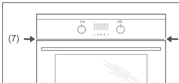
The external cooling fan is automatically switched on and off with the oven. It cools down the steam and vapour that exit the oven through the extractor (7) and prevents adjacent units from becoming too hot.
