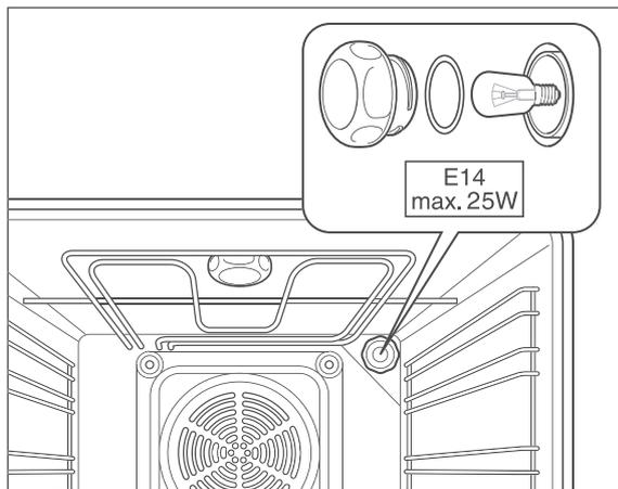
3. Unscrew the glass cover anticlockwise and remove it.
