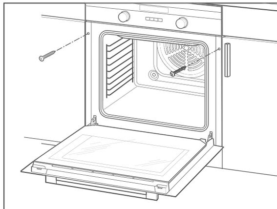
3. Once the oven is correctly positioned, open the oven door and screw into the unit using the fitting screws supplied.
