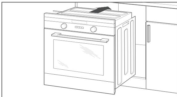
1. Push the oven into the recess until the front fascia is flush with the installation unit.
