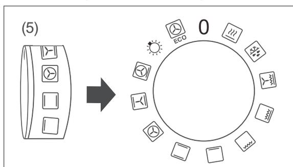
Use the function selector (5) to switch on the oven and select the heating method: The oven light and external cooling fan are switched on automatically. The power indicator light illuminates.
