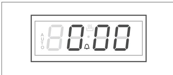
1. Press the MENU button until the display shows "0:00" and the bell symbol
