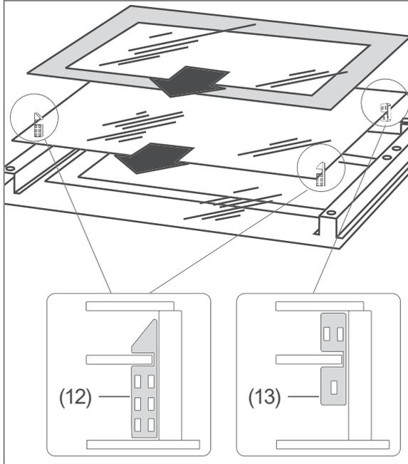
3. Remove the upper pane from the mounts below the hinges and carefully set it down.
