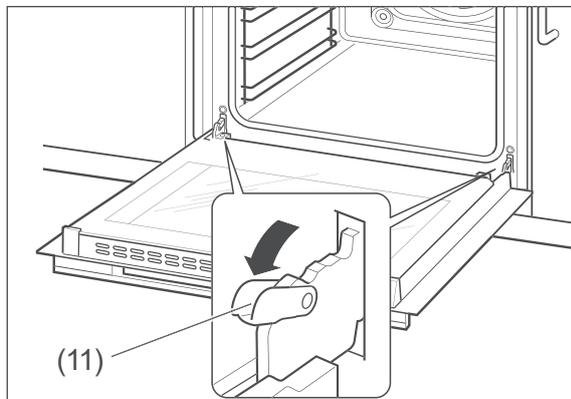
2. Fold the clips (11) on both sides all the way forward. Use a screwdriver if necessary.
