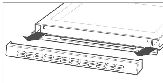
2. Carefully removed the metal grid.
