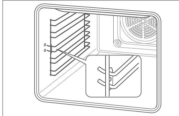
3. To remove the baking tray guides (8), first pull out the front holder on the front side, where the two hooks with the welded plates are situated. Then pull out the rear mount of the baking tray guides.
