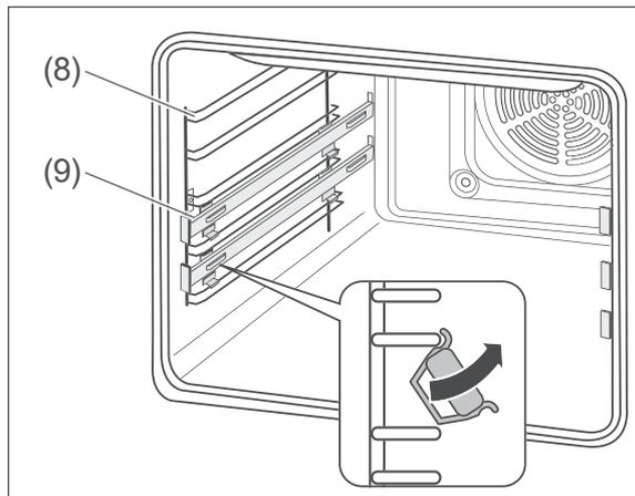
2. First pull the telescopic rails (9) off the lower guide of the oven rack guide (8) and then remove them by pulling upwards.
