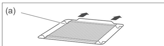
The supplied baking tray (b) and the dripping pan (c) both have an angled edge. Please ensure that this edge is facing forward on being placed in the oven. The grilling rack (a) must be inserted as shown.
