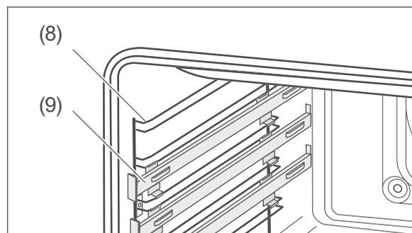
The side walls of the cooking compartment are equipped with baking tray guides (8) with telescopic oven rails (9). These make it easier to remove baking trays and the oven rack from the oven, for example, to baste roasts.
