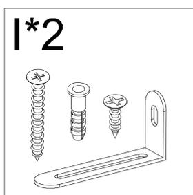
**⚠ Warning:** To keep safety, the cabinet has to be fixed to a wall with the anti-tipping accessories which are supplied.
