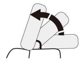
To move the headrest back to the flat position, first move it to the greatest angle possible, it will then fall back to the flat position.
