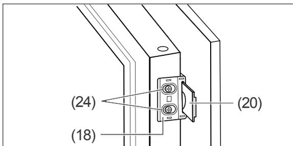
3. There are holes pre-drilled in the outside edges of the appliance door for the slides (18) to be attached. Use short screws (24) to attach 2 sliders each per door on the sides to be opened.
