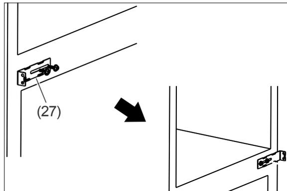
6. Detach the mounting bracket (27) and screw it back in on the opposite side.
