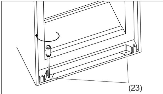
13. Once the doors open and close correctly, screw the refrigerating appliance to the built-in cabinet. To do so, use 3 short screws (24) at the top and the two long screws (23) at the bottom.
