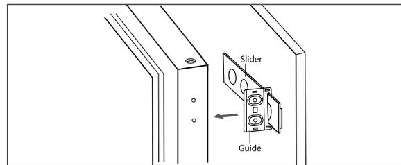
9. Unscrew the slides again and push them onto the fitted runners.
