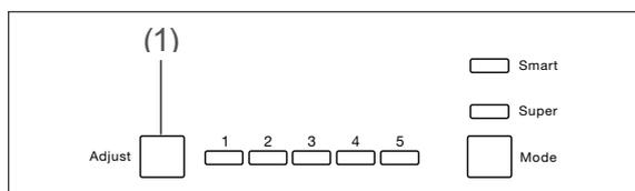
To switch the appliance off and on, press and hold the Adjust button (1) for 5 seconds.
