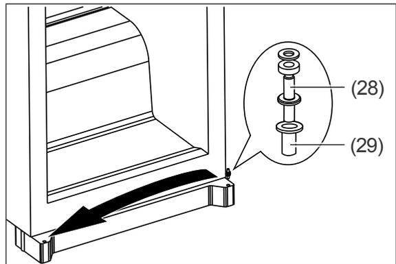
8. Transfer the lower hinge pin (28) over. Make sure that you also transfer over the sleeve (29) for the hinge pin.
