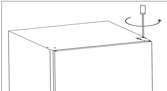
3. Remove the upper hinge plate. Use a size 8 spanner or a cross-headed screwdriver to remove the screws.
