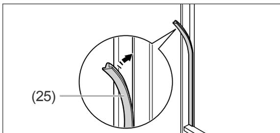
14. With the refrigerating appliance doors open, press the sealing strip into the gap between the cooling appliance and the built-in cabinet.
