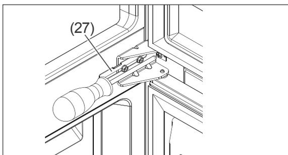
15. Finally, screw the two mounting brackets (27) between the upper and lower door with the built-in cupboard. Use the short screws (24) for this. Installation is now complete.
