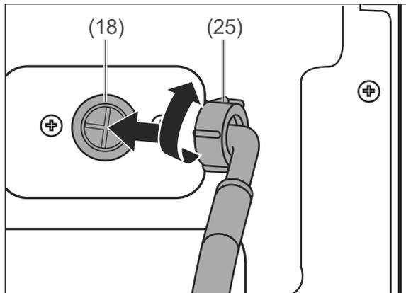
5. Unscrew the water inlet hose from the appliance.
