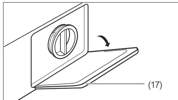
3. Carefully open the shutter (17) of the lint trap with a flat object, such as with a flat-tip screwdriver.
