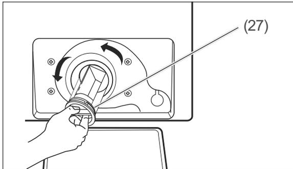
4. Place a suitable collecting container underneath the lint trap (27).
