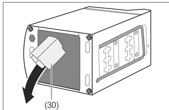
5. Carefully tilt the appliance on its side, and make sure that the styrofoam protector (30) is also removed. If it is still in the recess in the base of the appliance, remove it.
