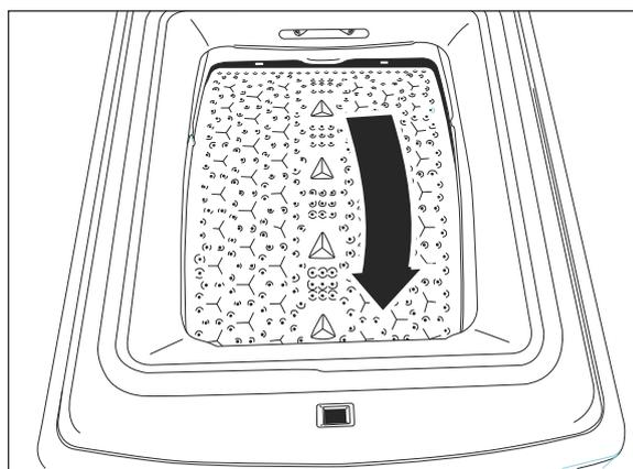
2. Turn the washing drum until the drum lock is up.
