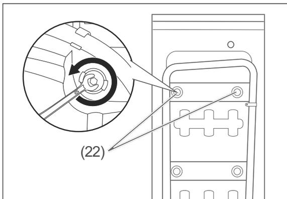
1. Loosen the screws of the transport safety devices (22) using a 10 mm wrench.
