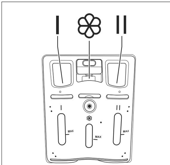
The dispenser (15) is located on the inside of the appliance lid and has three compartments:
