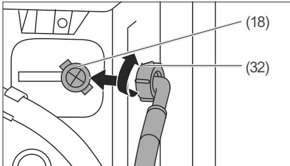
1. Screw the enclosed water inlet hose onto the connection (18) by hand. To do so, turn the union nut (32) clockwise.
