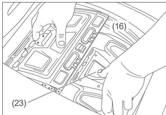
3. To open the washing drum (16), press the plastic tab (23) down slightly on the smaller section of the lid until the locking hooks disengage.
