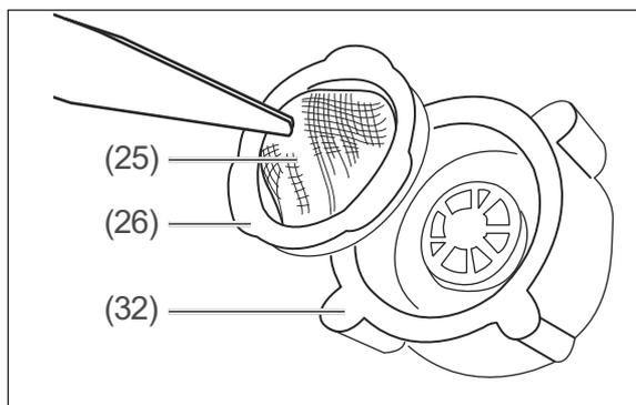
6. Use tweezers or a pair of pliers to pull the filter (25) with gasket (26) out of the union nut (32). Rinse the filter under fresh water and clean with a small, soft brush if necessary.
