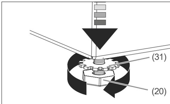
1. Loosen the lock nut (31) of one of the screw-on feet (20) underneath the appliance.
