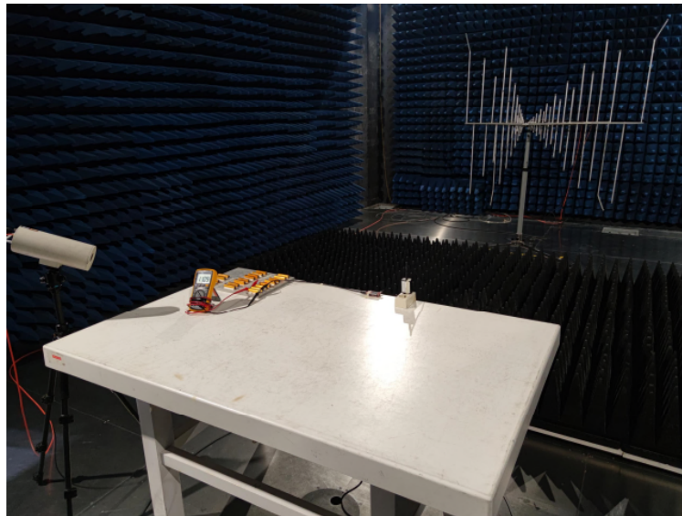
Photograph 5: Set-up for Radio-frequency Electromagnetic Fields (RS)
