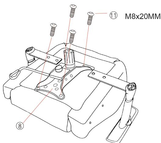
\*Tilt mechanism assembly sequence\*
