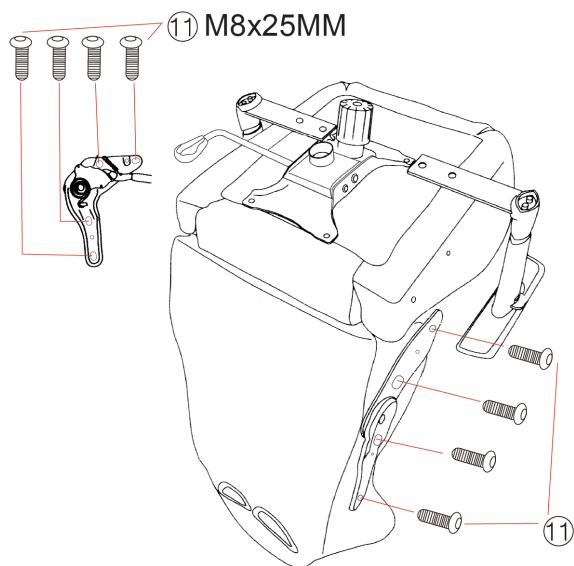
\*⑪ Screws have been assembled on the seat and backrest, please loosen them for further assembly.\*
