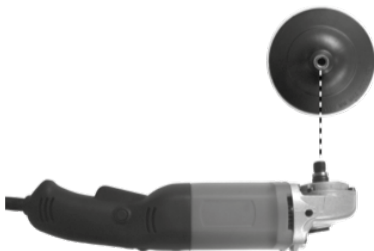
Figure 2: Installation of polishing plate
