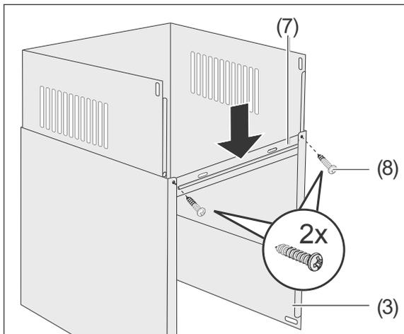
3. Place the retaining plate (7) onto the lower flue screen (3) so that it lines up with the chamfers on the inside. (Screws and elongated holes should point upwards).
