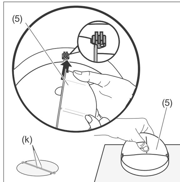
1. Place the two halves of the check valve (5) into the opening on the top of the Exhaust hood (1). Make sure that the pins (k) on the valve are facing outwards.
