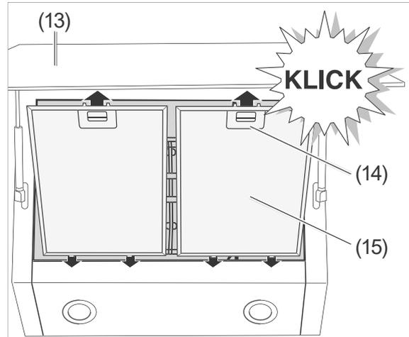
8. Place the grease filters (15) with the pins into the openings.
