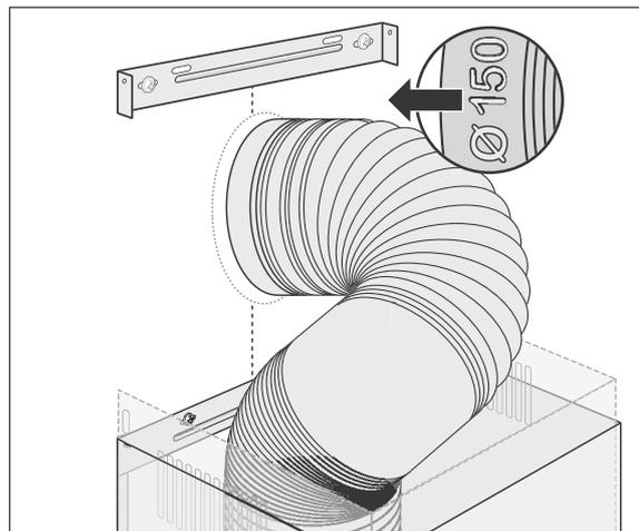
7. For exhaust air operation only: Insert the exhaust air hose (4) into the connection at the wall break (hose end with 150 mm diameter).
