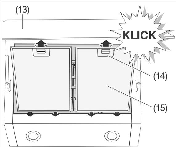
5. Place the grease filters (15) with the pins into the openings.
