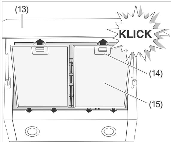
6. Place the grease filters (15) with the pins into the openings.
