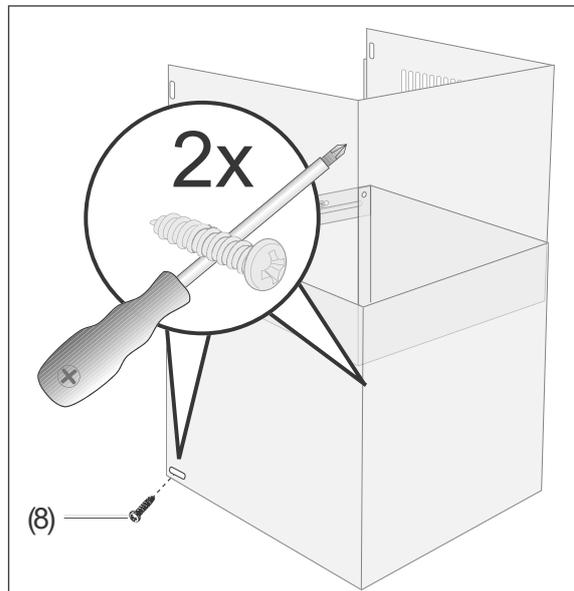
5. Place the entire flue screen onto the exhaust hood, with the closed side of the flue screen facing forward.
