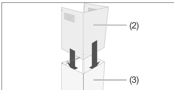
2. Push the upper part (2) of the flue screen halfway into the lower part (3) of the flue screen.
