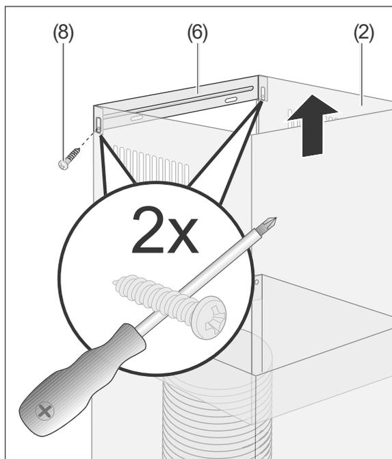
1. Pull the upper part of the flue screen (2) all the way up to the wall bracket for the upper flue screen (6).
