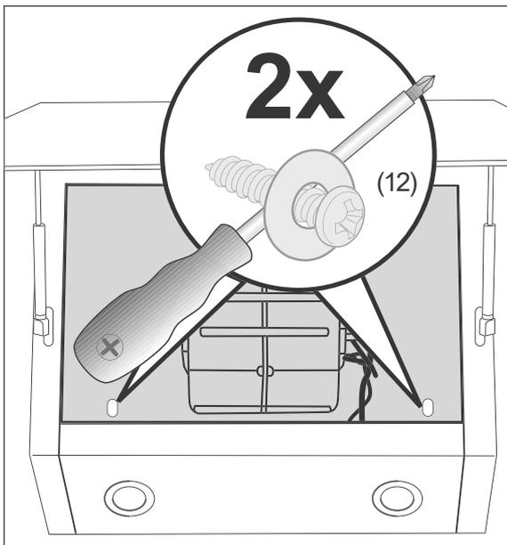
7. Turn two round-head screws (12) into the prepared wall plugs to secure the Exhaust hood, and screw the Exhaust hood tightly to the wall.
