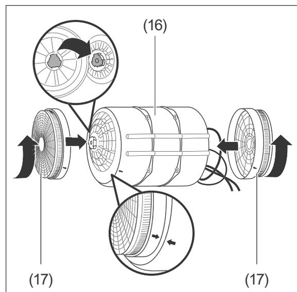
5. Place the new activated charcoal filters to the right and left of the motor and tighten them in an anti-clockwise direction. Allow the locks to click into place.
