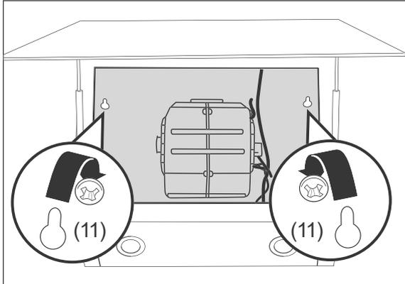
5. Carefully mount the Exhaust hood on the two round-head screws (11) on the keyhole openings.
