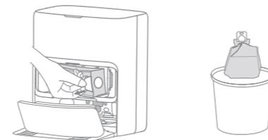
**Note:** Pulling outwards on the handle will seal the bag to prevent the dust and debris from accidentally falling out.
