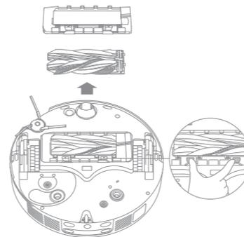
2. Pull out the brushes as shown in the figure. Use a proper cleaning tool to remove any hair tangled in the brush. After cleaning, push the brushes firmly into the main brush holder until they click into place.
