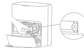
4. Reinstall the dust tank cover.
