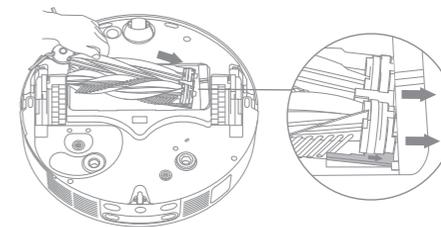
4. Align the front end of the brush guard with the slot, insert it downwards in an inclined way, and then press it into place.
