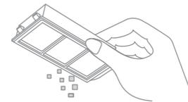
**Note:** Do not attempt to clean the filter with a brush, a finger or sharp objects to prevent damage.
