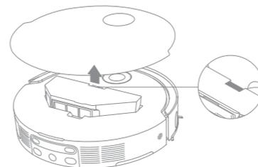
2. Remove the dust box filter, and then empty the dust box.
