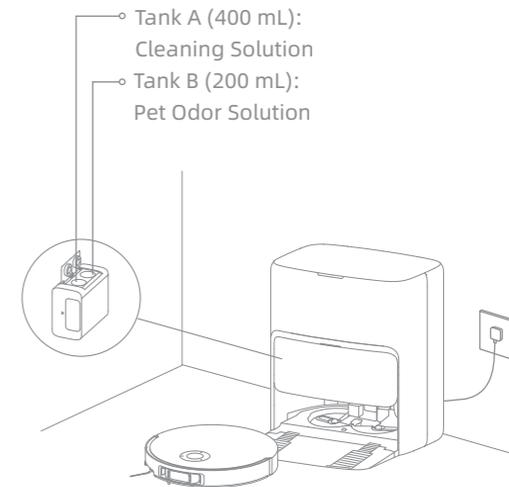
**Note:** Configure the auto solution dispenser module via app for different solution uses.
