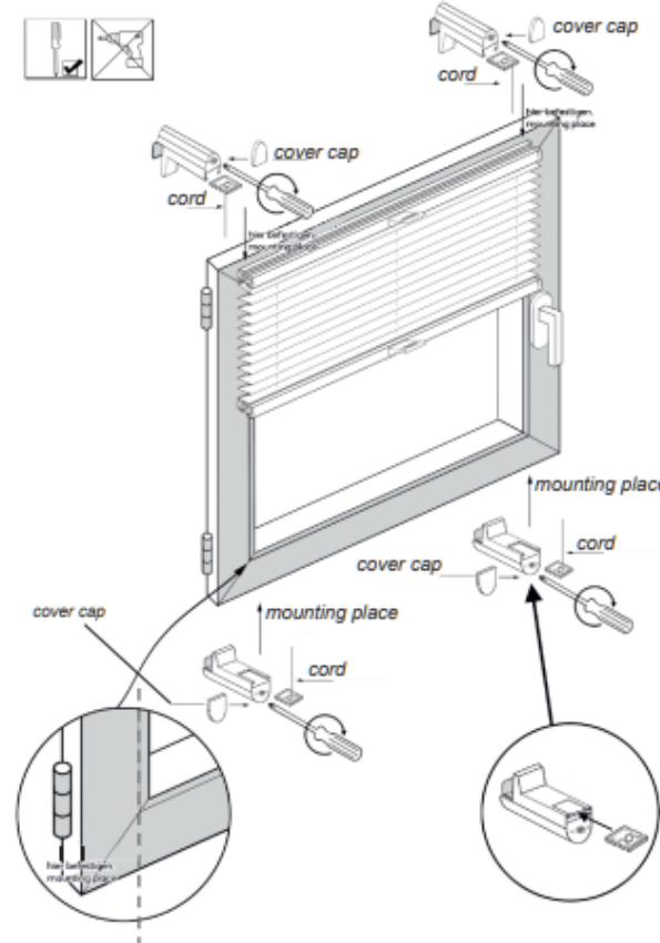
The clamp brackets are attached to the top and bottom of the open window.
