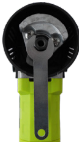
Figure 4: Place a wrench
