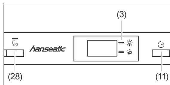
2. Press the  $\text{Q}_\square$  button (28) for 5 seconds within 60 seconds of switching on.
