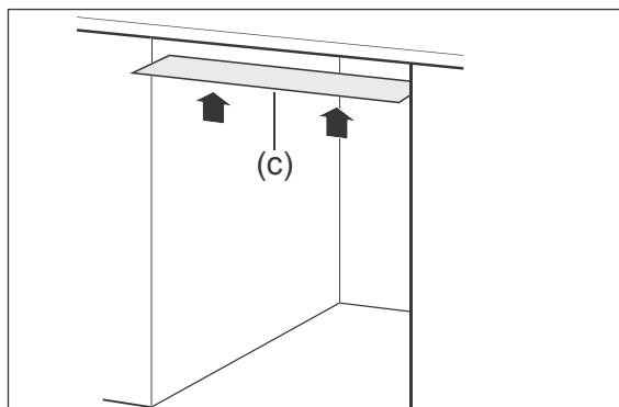
Affix the enclosed condensation-protective film (c) to the bottom of the work surface. In this way, you will avoid damage to the work surface as a result of hot steam which may be emitted from the dishwasher if the dishwasher door is left open.
