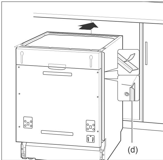
4. Remove the protective films from the side end profiles (d).
