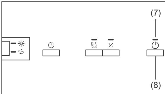
1. Open the dishwasher door and switch the dishwasher off using the button (8).
