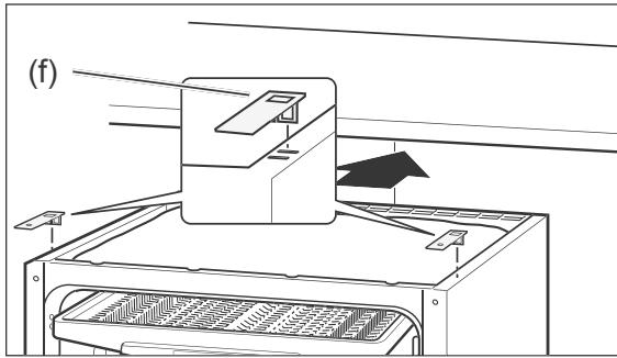
3. Insert the two mounting brackets (f) into the front slots on the top of the dishwasher so that you can screw the dishwasher to the worktop subsequently.
