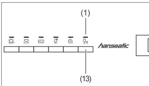
2. Press and hold the (13) button for as long as required until the display shows the current water hardness (H 1 to H 5).
