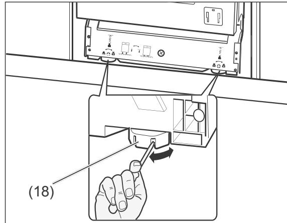
7. To position the dishwasher so that it is level, the two front adjustable feet (18) and the back foot on the appliance can be adjusted by up to 50 mm.
