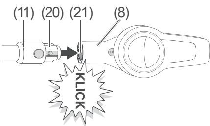
2. Insert the connector (20) on the tube extension (11) into the opening (21) on the suction tube (8).
