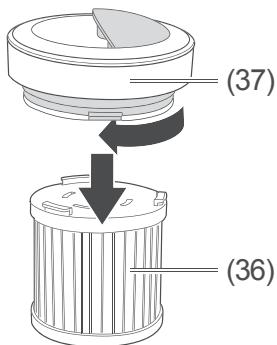
6. Reattach the filter cover (37) to the hygiene filter (36) and turn it **clockwise** to tighten it.
