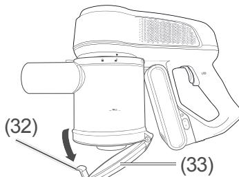
3. Press the locking button (32) on the base of the dust bin (33). The base of the dust bin (33) opens out downwards and the dust falls into the waste bin.
