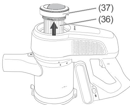
2. Lift out the hygiene filter (36) on the filter cover (37).
