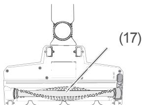
The rotating brush (17) is propelled by the vacuum air flow. It is particularly suitable for vacuuming hair and thread from rugs and carpeted floors.
