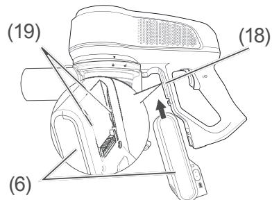
1. Insert the battery (6) onto the handle of the appliance. Make sure that the guide rails (18) on the appliance slide into the guide rails (19) on the battery (6).
