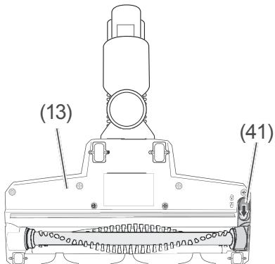
2. Move the slider (41) on the underside of the floor nozzle (13) to the "Open" position (towards the
