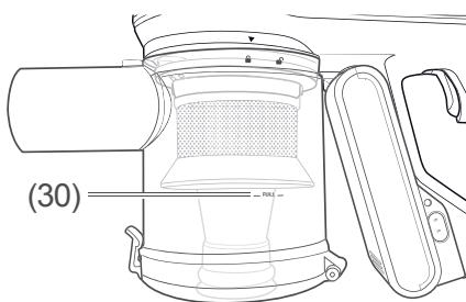
You should empty the dust bin at the latest when the dust in the dust bin reaches the "Full" mark (30).
