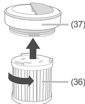
3. Turn the filter cover (37) **anticlockwise** and pull it off the hygiene filter (36).
