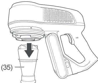
6. Remove the suction piece (35) and wash it under running water.
