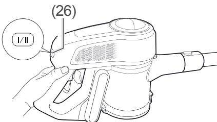
The appliance is equipped with two suction levels. Set the suction level using the suction level switch (26).
