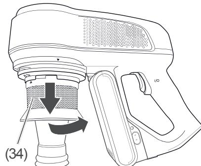
4. Turn the dust bin (34) **anticlockwise** until the
