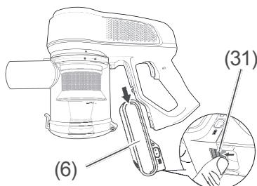
1. First remove the battery (6). To do this, press the locking mechanism (31) on the battery (6).
