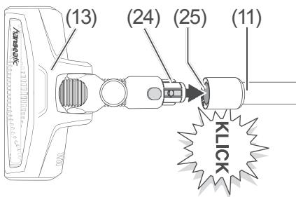
3. Select a nozzle, e.g. the floor nozzle (13), and insert the connector (24) of the floor nozzle (13) into the opening (25) on the tube extension (11). Make sure that the connector pins (22) slide into the openings (23).
