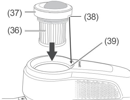
7. Reinsert the hygiene filter (36) with the filter cover (37). In doing so, make sure that the recess (37) in the filter cover (38) hooks into the lug (39) on the appliance housing.
