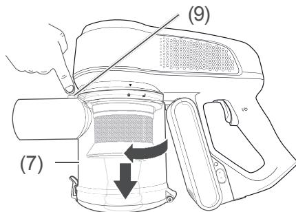
2. Press the release button (9) for the dust bin (7).
