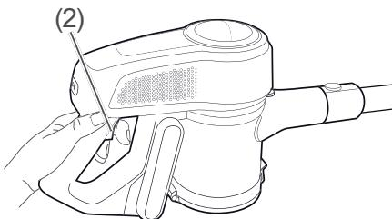
1. Press the On/Off switch (2) to turn the appliance on.
