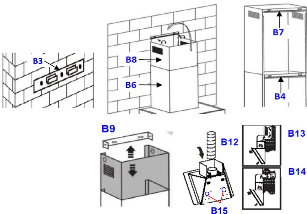
12. Fix the exhaust hose **B12** on its final position according to **B13** or **B14**.
