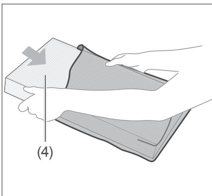
3. Remove the hygiene filter (4) from the protective cover.
