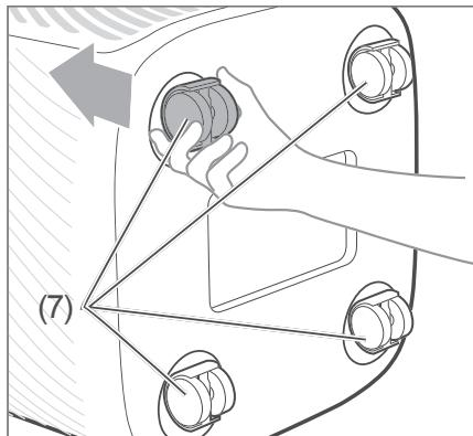
8. Place the device on its side and attach the castors (7).
