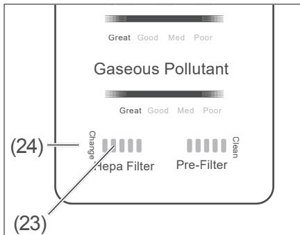
During the life cycle of the hygiene filter, the bars shown on the lifetime display (23) will go out one after the other. When the last bar turns red and the "Change" (24) display lights up, you should replace the hygiene filter.
