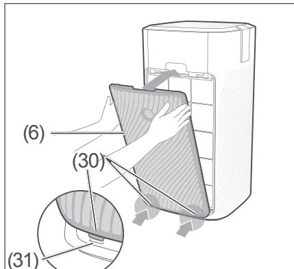
3. Replace the filter cover (6). Make sure that the connector pins (30) slide into the openings (31).
