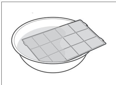
If the prefilter (5) is very dirty, you can soak it in a normal detergent solution for 10 minutes and then carefully clean it with a brush. Then leave the prefilter to **dry out completely** before reinserting it.
