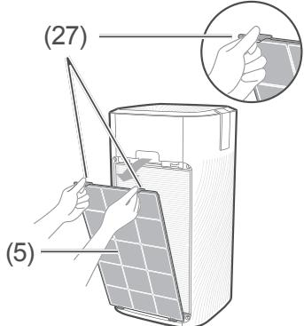
2. Remove the prefilter (5). To do this, please press the unlocking buttons (27).
