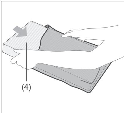
4. Remove the hygiene filter (4) from the protective cover.
