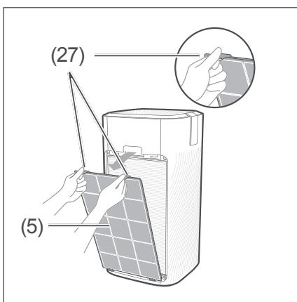
3. Remove the prefilter (5). To do this, please press the unlocking buttons (27).
