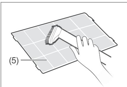
4. Clean the prefilter (5) either with a brush by brushing sideways over the filter or with the vacuum cleaner.
