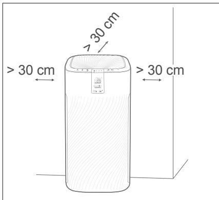
1. Set up the appliance so that there is a gap of at least 30 cm on either side and to the wall.
