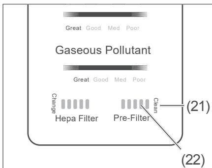
Over the course of time, the bars on the pollutant indicator (22) for the prefilter will go out one after the other. When the last bar turns red and the "Clean" (21) indicator lights up, you should clean the prefilter.
