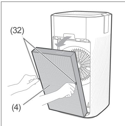
2. Remove the hygiene filter (4). To do so, pull on the strips (32).
