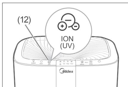
8. Press the ION button (12) for approx. 3 seconds to reset the filter.
